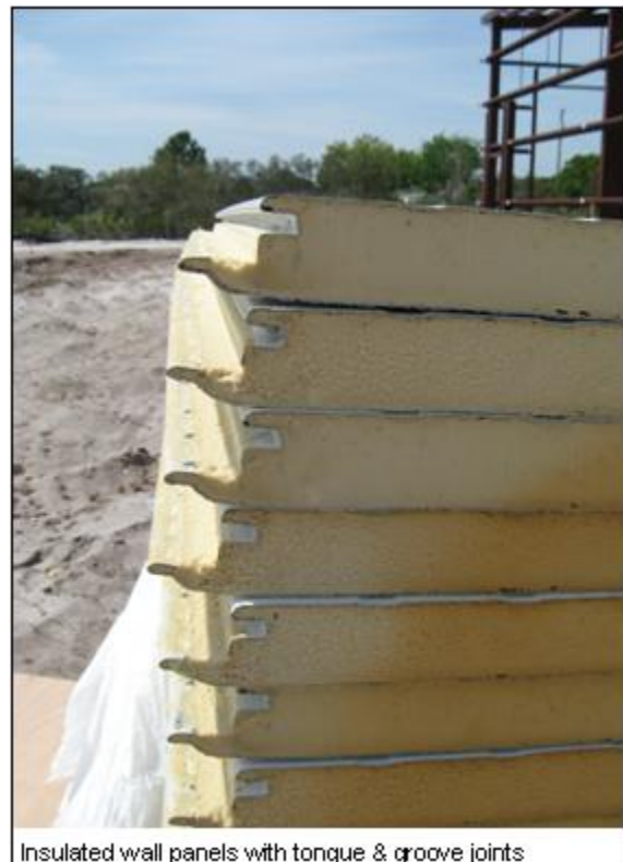
Insulated wall panels with tongue & groove joints
